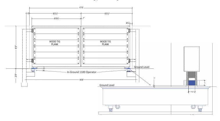
When installed, the center of the pivot pin of the operator must be installed directly in line with the center of the gate hinge to prevent binding.
